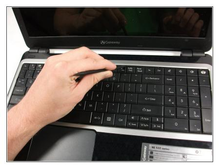
• Take the plastic spudger and pull up the tabs on all four sides of the keyboard molding.
