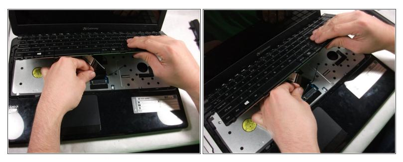
• Carefully unplug the ribbon cable attached to the motherboard.
