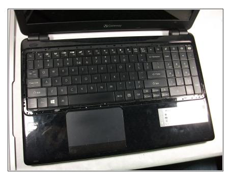
Carefully lift the keyboard molding out.
