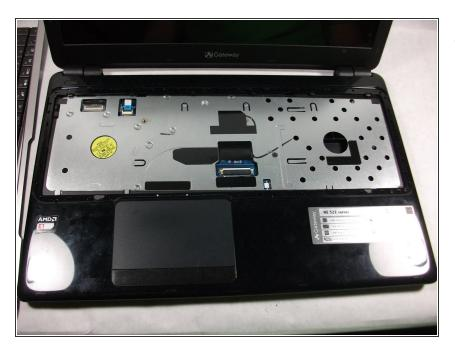
• Lift and remove the keyboard from the computer.
