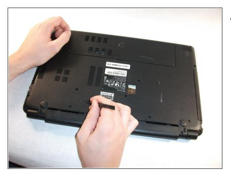
• Either using your fingers or a plastic spudger push the battery clip to the left to release battery.
