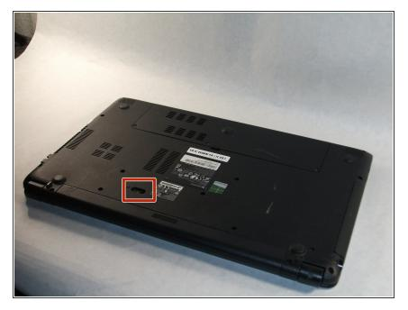
Make sure the laptop is turned off and flipped over so that the bottom is facing up. Then, locate the battery clip as shown.
