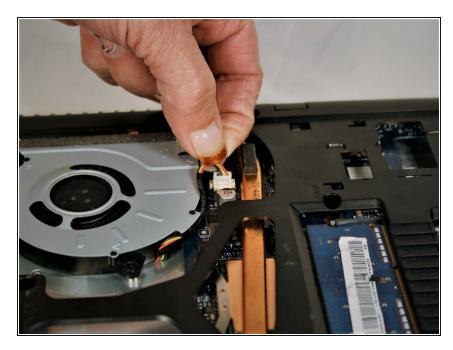
• Disconnect the fan wires from the motherboard by lifting upwards
