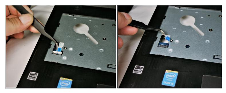
• lift clip to remove power button ribbon cable.
