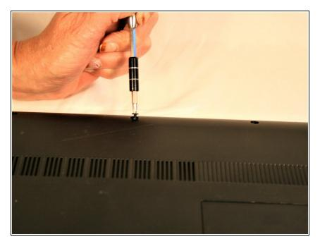
Remove screws using a 001 phillips screw driver.
