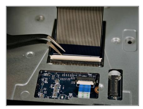
• Using tweezers, lift up clip to remove keyboard ribbon cable.
