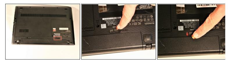
• Slide the tab positioned on the right side to the right.
