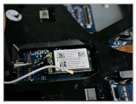
• Remove wifi wires by lifting up
