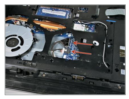
• locate power and monitor cable on bottom side next to fan
