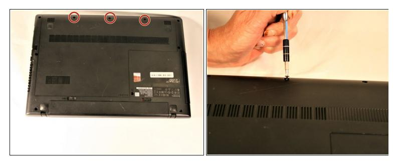
Remove the three screws securing the outer cover of the laptop using a Phillips #0 screwdriver.
