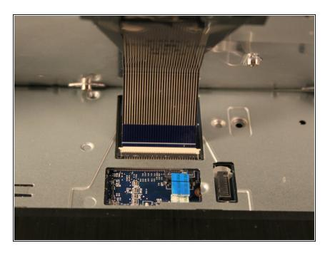
lift up bottom of keyboard slightly, to access keyboard ribbon
