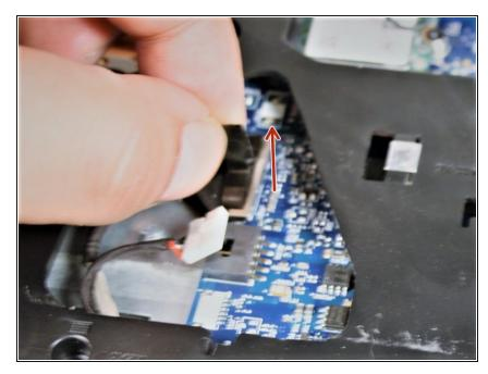
• remove monitor cable by gently pulling on tab straight up
