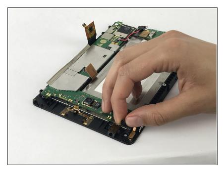
Once the battery is removed, remove the front facing camera from the socket located on the top left of the tablet.
