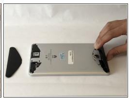
Use either your finger or a metal spudger to lift both the top and bottom black covers on the back of the tablet.
