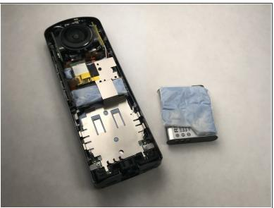
• Lift the battery out of the device, beginning with the end closest to the camera.
