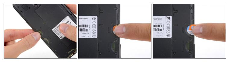
• Push to eject and remove the MicroSD and SIM cards (if installed).
