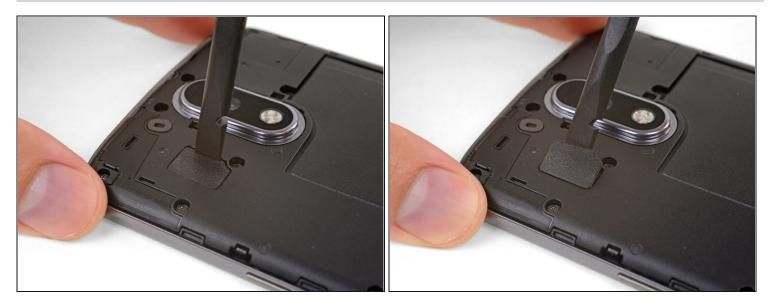
• Use a spudger to pry up the rubber cover for the camera flash connector.
