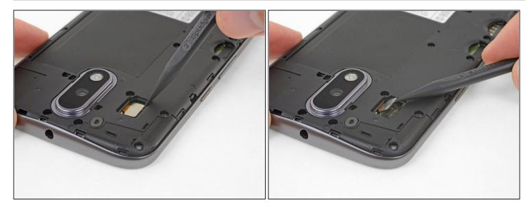
• Use a spudger to disconnect the camera flash connector by prying it straight up.
