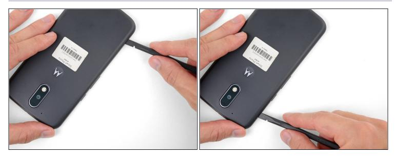
• Slide your tool all along the side of the phone to separate more of the clips securing the back cover.
