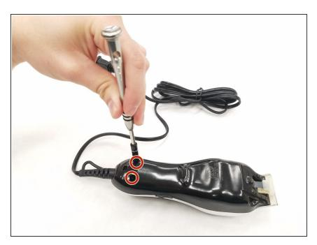
Remove the two 12.0 mm JIS #1 screws on the back of the device body.
