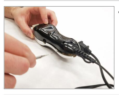
Pry the body case off of the device using a spudger.
