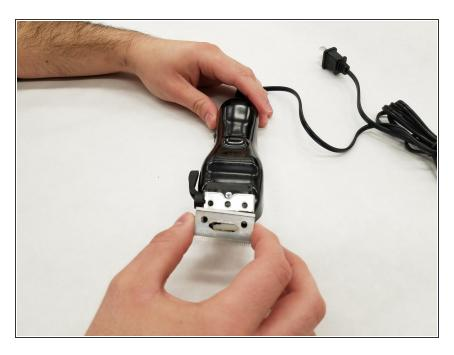
Lift the bottom blade straight up from the device body to remove it.
