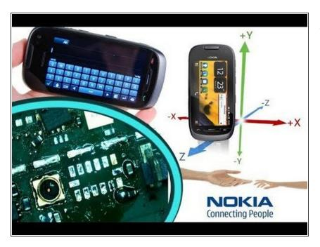
To fix the accelometer watch the video carefully. This sensor is responsible for the screen rotation.
