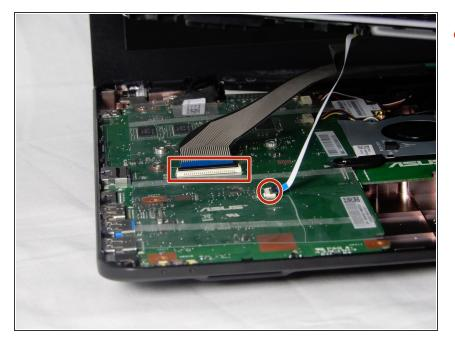
Observe where the ribbons connect to the motherboard, there are two connections. Each connection has a black clamp. To remove the ribbon, lift the black clamp up to disconnect it.
