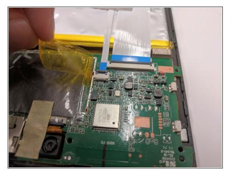
Carefully peel off the tape covering the circuit boards and blue ribbons. The tape can be disposed or saved for reuse.
