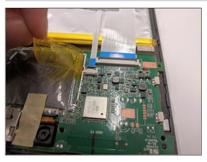
Carefully peel off the tape covering the circuit boards and blue ribbons. The tape can be disposed or saved for reuse.
