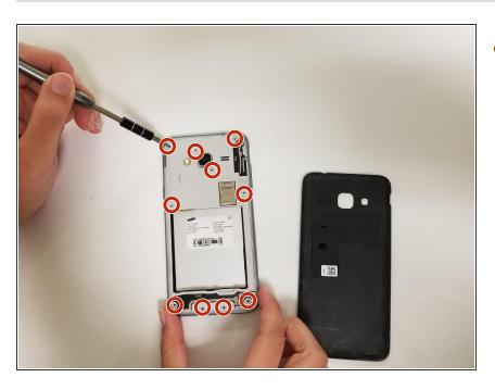
Remove all ten screws by using a Phillips #000 screwdriver.
