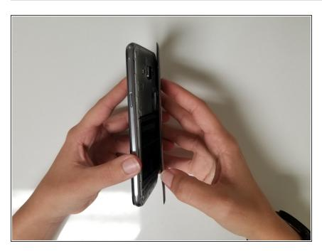
Separate the back casing from the phone by carefully using your fingers to pry them apart.
