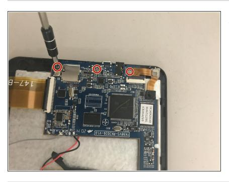
Use the Phillips #0 screwdriver to remove the three 1 mm screws from the motherboard.
