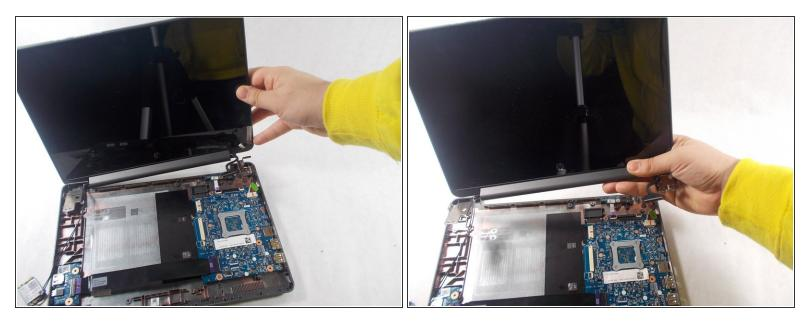
A Be careful when removing the screen so it doesn't get caught on any wires.
