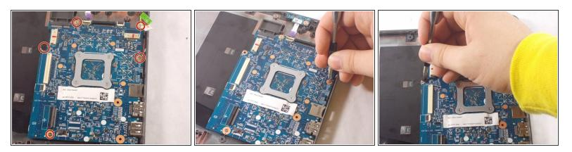
• Use a Phillips #0 screwdriver to remove five 1.3mm screws that hold the motherboard in place.
