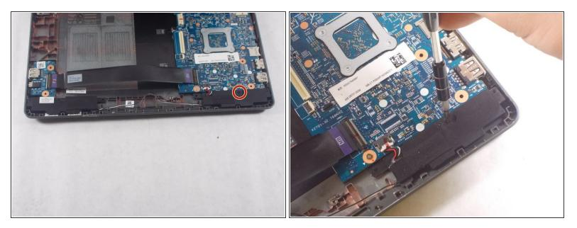
Use a Phillips #0 screwdriver to remove the one 1.3mm screw that connects the speakers and the motherboard together.
