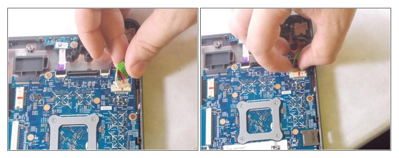
A Please hold the white tab and not the wires or it may rip the wires out.
