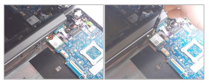
Use a Phillips #0 screwdriver to remove the 1.3 mm screw that holds the wireless card.
