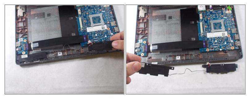
A Be careful with the wire between both end of the speakers. It's between metal parts and can get caught.
