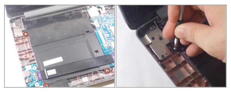
• Remove three of the 1.3mm screws that keep the battery in place with a Phillips #0 screwdriver.
