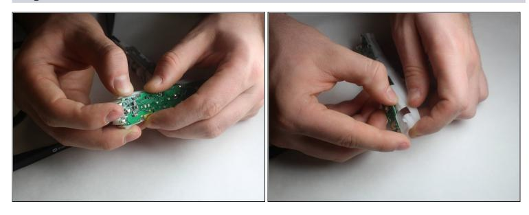
• All points of contact between the mother board and the other components should now be de-soldered. Remove the motherboard by gently pushing up on it, pulling it out of the plastic tabs that secure it to the housing.
