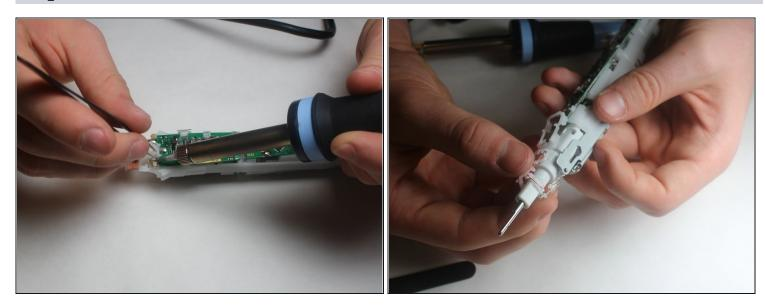
• Use a pair of <u>tweezers</u> to remove the plastic housing and the LED from the device.
