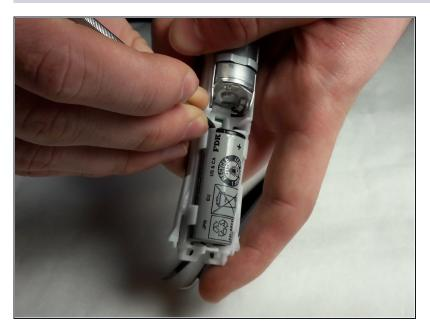
Use a metal spudger to pop the battery out of its casing. The electrodes will remain attached to the battery.
