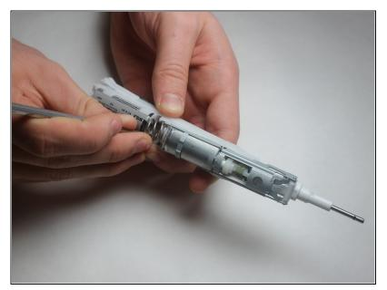
Remove the spring from the housing using a nylon spudger.
