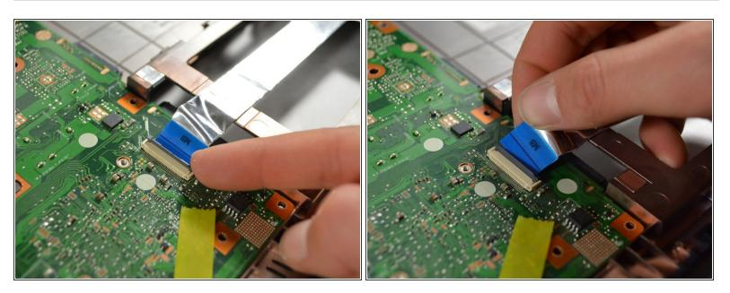
• Remove the blue cable on the bottom right by lifting up on the tab and pulling the cable out.
