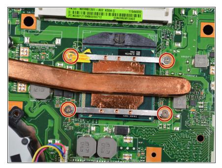
Remove the four 2 mm Phillips head screws surrounding the copper rod using PH1 screw driver.
