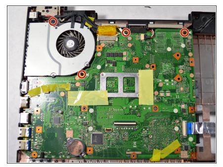
Remove the four 2 mm Phillips head screws from the top of the motherboard and fan using PH #1 screwdriver.
