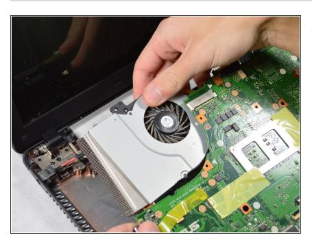
Slide the fan out from the ridged metal component.
