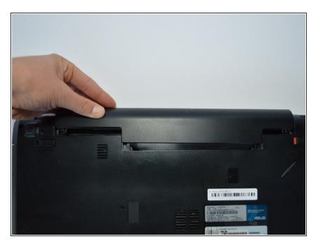
Gently slide the battery out while still holding the left unlock switch.
