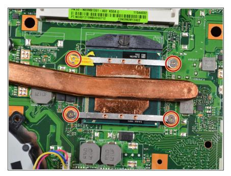
Remove the four 2 mm Phillips head screws surrounding the copper rod using PH1 screw driver.
