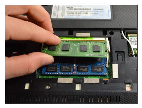
Remove the RAM by lifting up with your fingers and sliding it out towards you.
