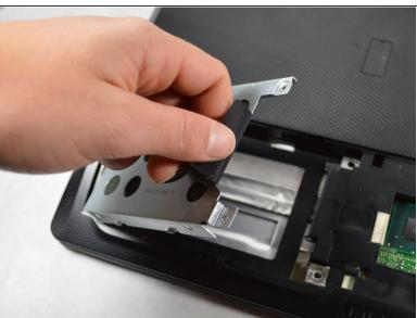
Remove the hard drive by sliding it to the left and lifting up.
