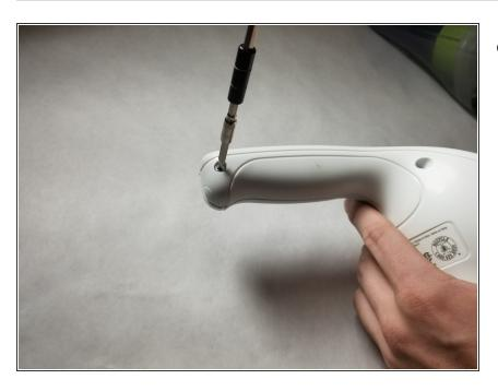
Unscrew and remove all 5 screws using the Phillips 0 screw bit. Each screw is 17.5 mm long.
