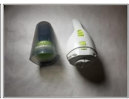
To remove the filter and housing, press the green button labeled "Filter".
