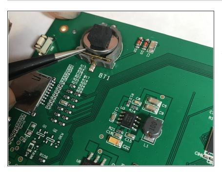
The battery can then be popped out using precision tweezers and replaced with a new one. To reassemble your device, follow these instructions in reverse order.
