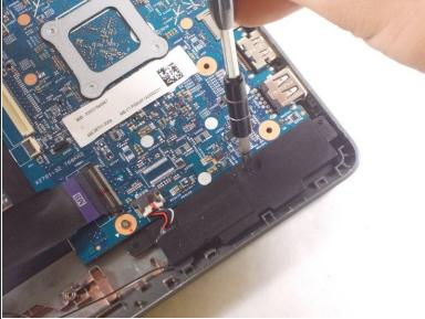
Use a Phillips #0 screwdriver to remove the one 1.3mm screw that connects the speakers and the motherboard together.
