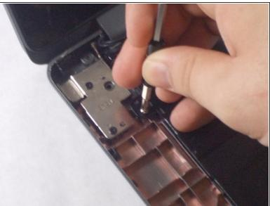
Remove three of the 1.3mm screws that keep the battery in place with a Phillips #0 screwdriver.
