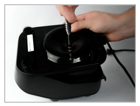
Remove six screws (12mm long, 6mm head diameter) from bottom of the blender using a Phillips #2 screwdriver
