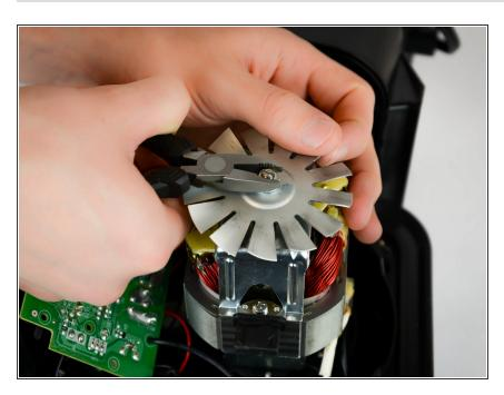
Using a needle nose pliers, remove nut holding fan in-place. Be careful with fan blades and use a glove or a thick cloth to protect hands.
