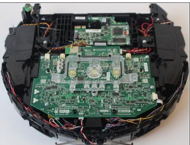
Lift the top plate slowly, being careful not to damage the vacuum components while exposing the motherboard.
