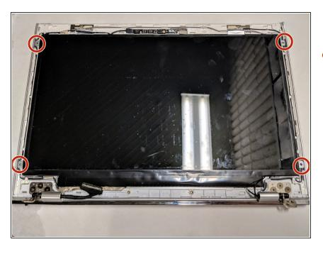
Unscrew the four 3mm Phillips head screws that secure the display to the plastic frame.
