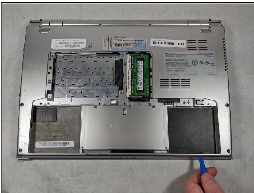
**⚠** Be careful when prying the back panel away from the laptop, the plastic frame and hinges that attach it to the back panel are prone to bending/cracking.
