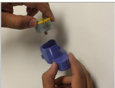
Remove the motor from the blue casing.
