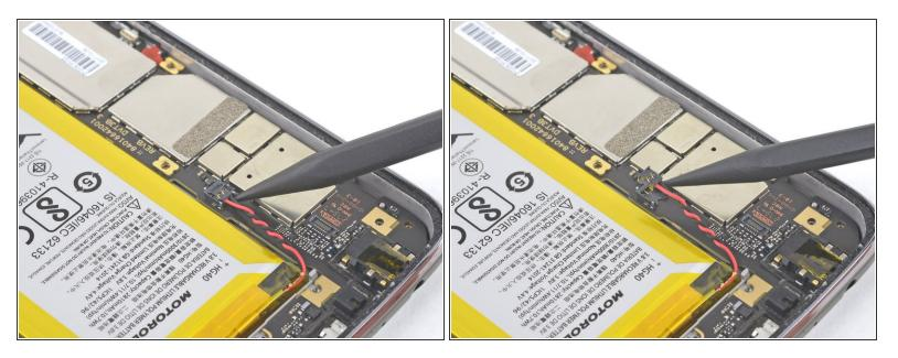
• Use the point of a spudger to disconnect the battery by prying its connector straight up from the motherboard.
