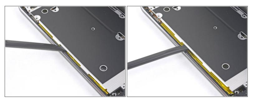
Insert the flat end of a spudger between the midframe and the left edge of the phone and carefully pry to release the two clips holding the midframe in place.
