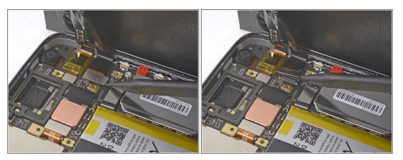
Use the point of a spudger to disconnect the larger of the two display cable connectors.
