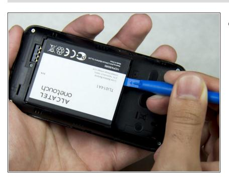
Using a plastic opening tool if necessary, remove the battery from the device.
