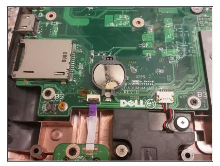
Use a plastic spudger to get under the CR2032 cell and pry it out carefully.
