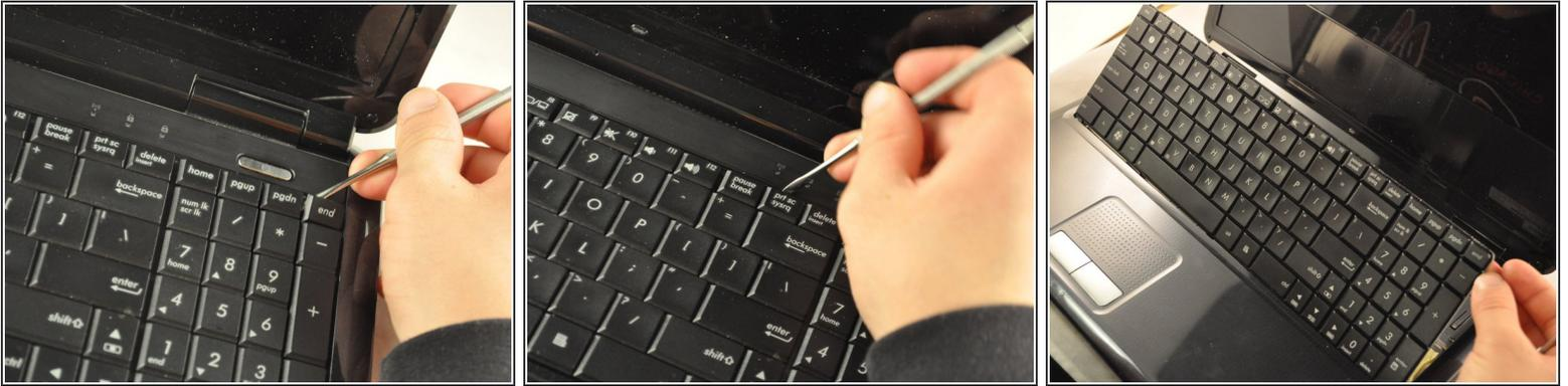
**⚠** The ribbon cable that was plugged into the motherboard is attached to the keyboard. Be sure not to damage it.
