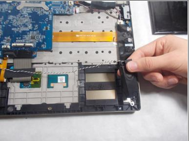
Carefully pull both the left and right speaker modules out of the computer.
