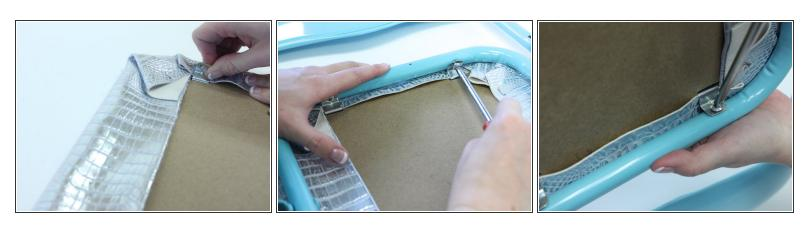
Insert the hinges into chair seat. Place the screw into the hinge, and then screw the chair frame to the chair seat. We found it helpful to have another person hold the chair frame while another person screwed the screws in.
