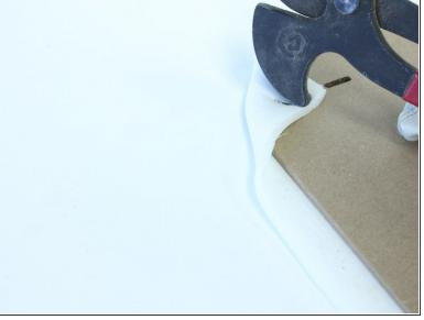
With proper safety attire including gloves and safety goggles attach the padding to the seat with staple gun. Using a tongue-grove pliers gently hammer the staples all the way into the padded seat.
