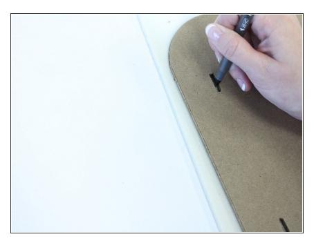
Inserts slits in the padding where the hinges will attach the seat to the chair frame.
