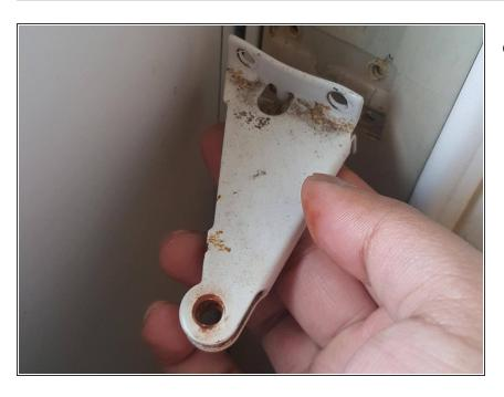
Loosen the screws from the door jamb bracket and remove.
