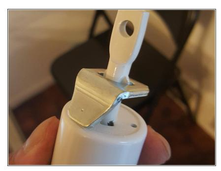
Slide the new clip (metal washer that was provided with the door closer) on the door closer barrel with the dented side facing inwards (as shown in photo).
