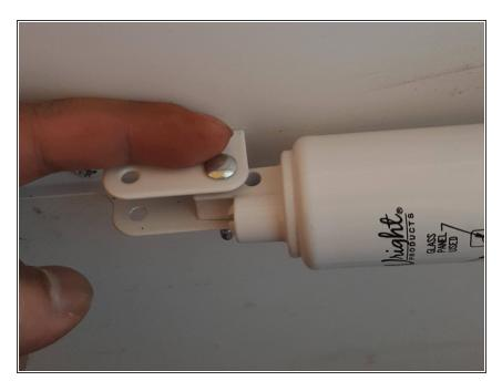
Slip the other pin into the barrel and the bracket.
