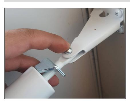
Insert the pin into the closer barrel and the jamb bracket.
