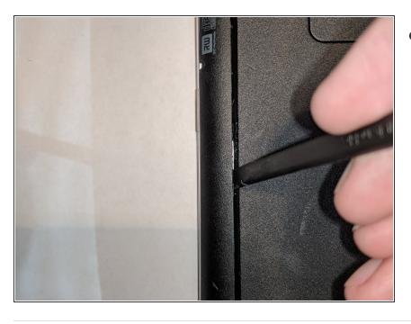
Using the spudger carefully place the pointed end into the gap that covers the optical drive.
