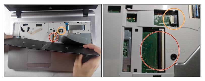
Once keyboard is removed, there will be two ribbon cables connecting the keyboard to the laptop. there will be two latches holding the cables in place on the laptop. to undo these latches, insert a spudger underneath the latch and lift up to free the cable.
