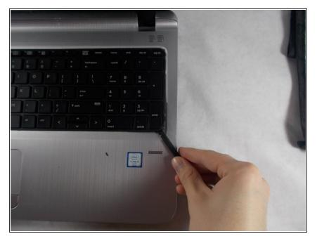
To remove the keyboard, gently insert the spudger underneath it along an edge and work it around to unsnap
