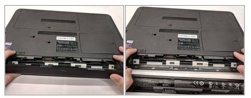
• Once the releases are in position, pull the battery out.
