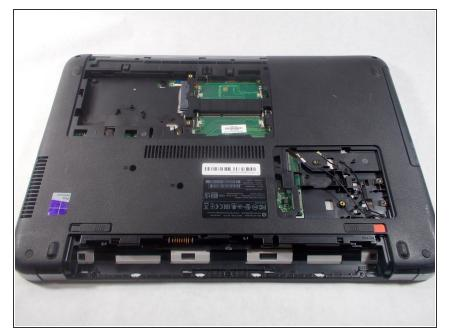
Once all of the Phillips 00 screws are removed, use a spudger to remove the four rubber stops in each corner. Underneath, there will be four Torx bit 8 size 5mm screws that need to be removed.
