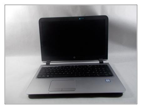
Once all of the screws on the bottom are removed, flip your laptop over and open it so the keyboard is visible.
