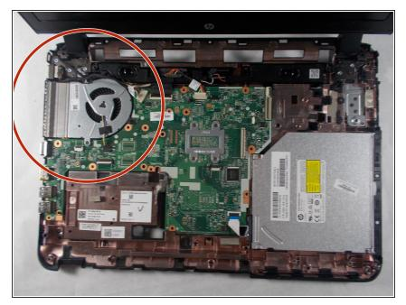
• Once the top part of the case is removed, you can access the fan, as well as other internal parts.
