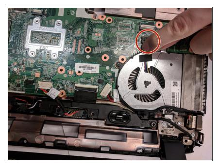
• To remove the fan, begin by unlatching this cable, as you did in step 3.
