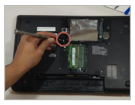
Unscrew the 2mm PH#1 screw next to the Toshiba Device information tag.
