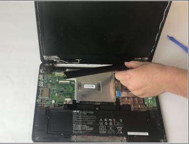
• Use plastic opening tool to remove plastic hinge casing located between the screen and keyboard.
