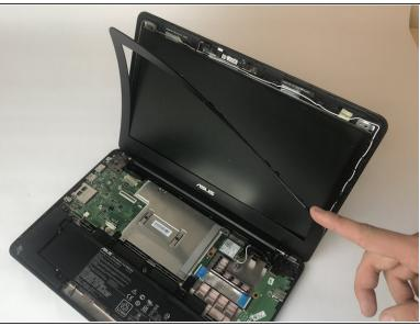
Use plastic opening tool to remove the frame around the screen. It is recommended to start in the upper corners.
