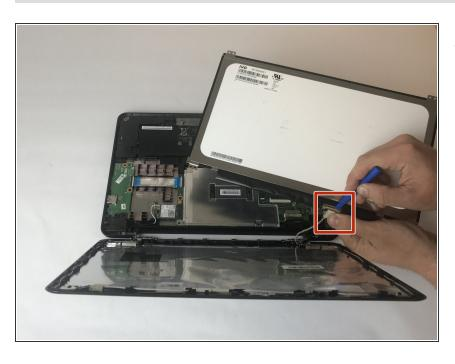
Use plastic prying tool to detach the wire that connects the screen to the lower non-display half of the laptop.
