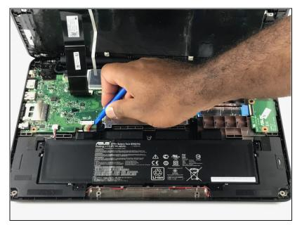
Unplug the wire using the plastic opening tool that connects the battery with the board.
