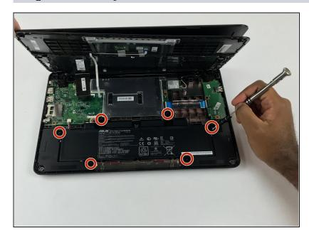
• Remove the six 6.0mm Philips screws, using the 64 bit driver from around the battery.
