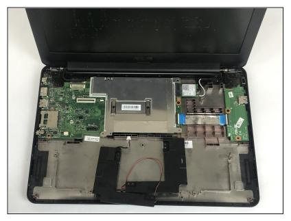
• Lift and remove both speakers and connecting wire.
