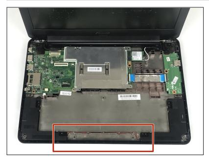
⚠ Gently remove the wire connecting the left and right speakers from it's channel. Be careful as to not tear or damage the wire.
