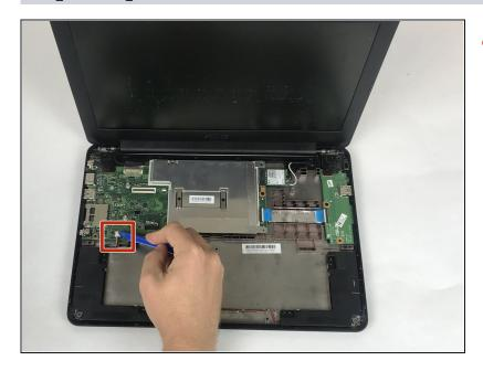
Use plastic opening tool to pry off the wire connecting the left side speaker to the circuit board.
