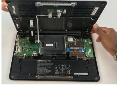
Lift the keyboard panel away from the components at its hinges, which are located at the back of the laptop.
