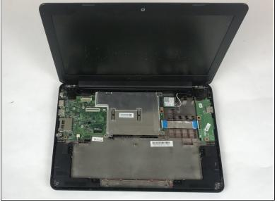
Lift and remove keyboard from device. The keyboard and Mouse pad are one part that must be replaced simultaneously.
