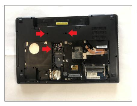
Unscrew the 3 "keyboard" detected screws.
