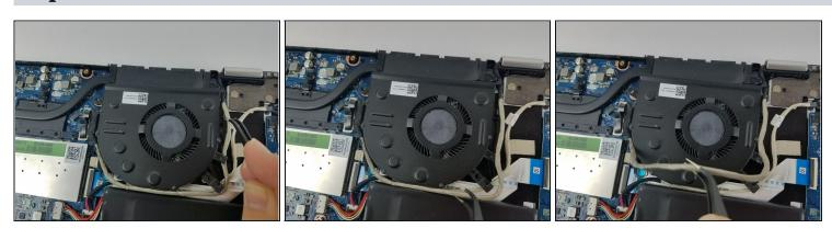
• Using the Precision <u>Tweezers</u>, remove the 2 gray wires around the fan from their clips.
