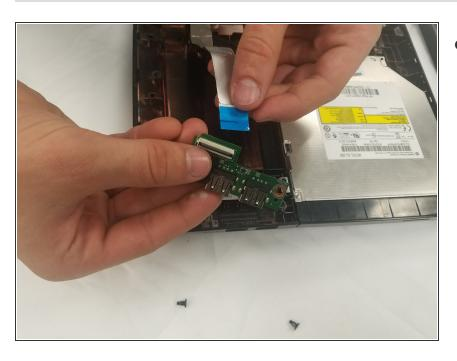
Next disconnect the flat cable by pulling the cable straight out of the connector from the USB Hub.
