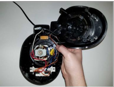
Remove the back panel using a Phillips #1 Screwdriver on the four screws that hold it in place.
