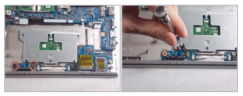
Unscrew the two 2mm screws from the board using JIS #0 screwdriver.
