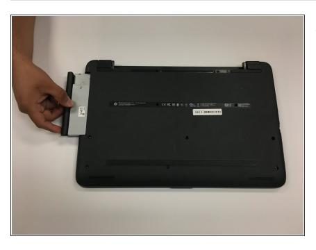
Locate the optical disc drive and remove it from the device by sliding it straight of the device.
