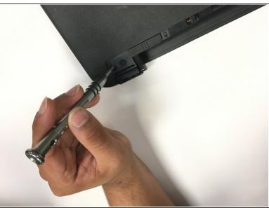
• In the same spot you've just removed the bumpers from, you will find two 5/16 in. screws. Using the same Phillips-head screwdriver used in step 2, remove the screws
