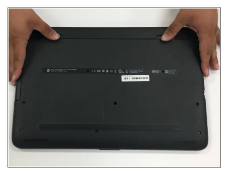
Slide the two battery lock latches on the back of the device to the "unlock" position.
