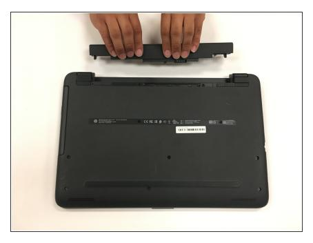
Lift the battery upward to remove it from the device.
