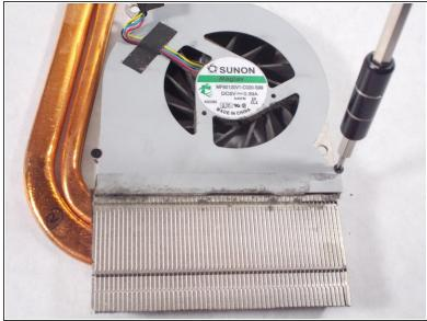
• Remove (2) 2mm screws on the sides of the cooling fan with a #00 Phillips screwdriver.
