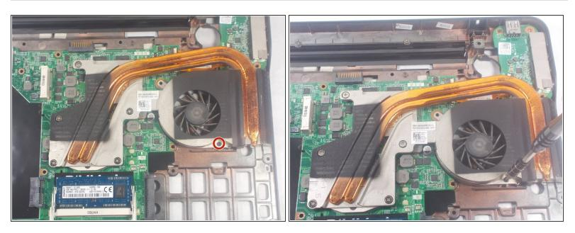
• Use a JIS 1 screwdriver to remove (1) 4mm screw on the cooling fan assembly.
