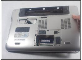
Separate the bottom cover from the top cover with plastic prying tool and finish lifting the bottom cover off.
