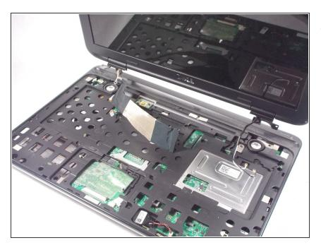
Lift the display assembly up and off of the main body of the laptop.
