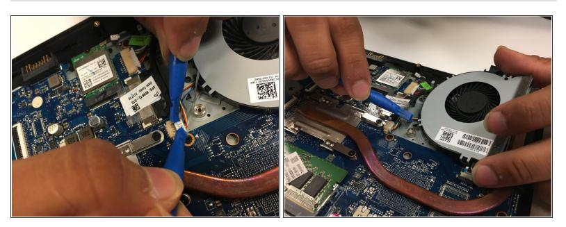
Use your fingers or tweezers to pinch both sides of the connector and remove the fan from the device.
