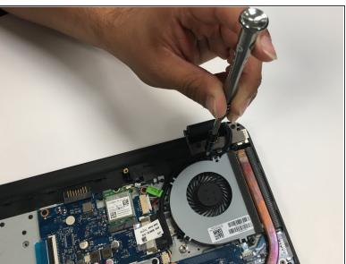
There are two 5/16 in. screws adjacent from each other that secure the fan to the device. Use the PH1 phillips-head screwdriver to remove them.
