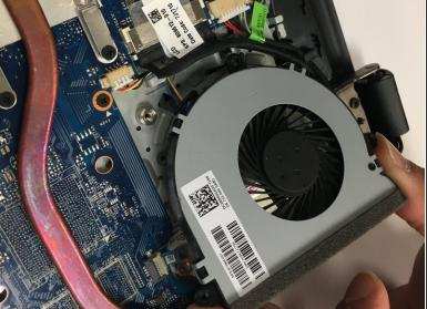
Lift the clear plastic strip holding down the fan and lift the fan out of place.
