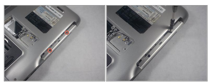
Remove two 4.5mm screws with JIS 1 screwdriver marked by the letter "K" in the optical drive bay.
