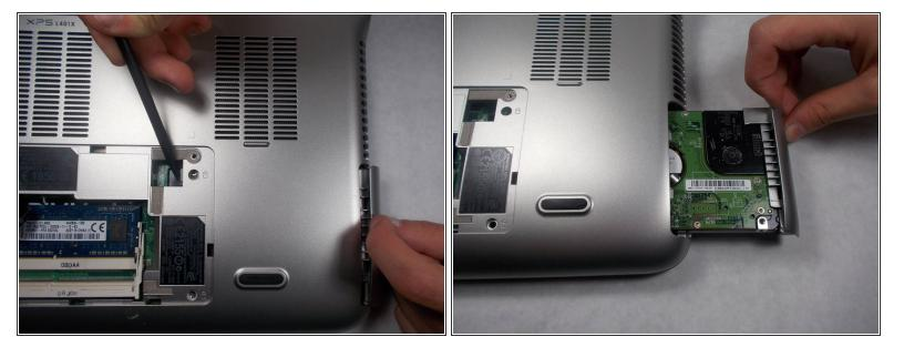
Push the hard drive to the right with a spudger to unseat it from its socket while pulling out the hard drive with your other hand.
