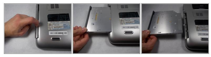
Carefully pull out the optical drive from its bay.
