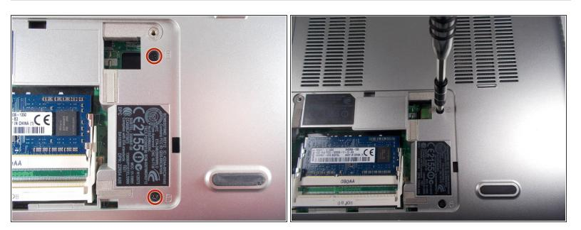
Use a JIS 1 screwdriver to remove (2) 2.5mm screws located on the right side of the RAM bay.
