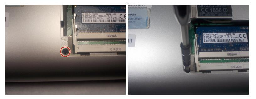
• Remove (1) 7.5mm screw with JIS 1 screwdriver marked by the letter "K" in the RAM bay.
