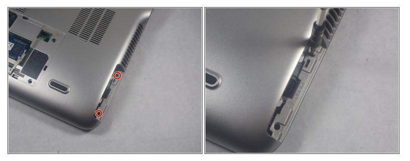
• Remove (2) 4.5mm screws with JIS 1 screwdriver marked by the letter "K"in the hard drive bay.
