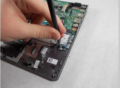
• Remove the single 3.0mm screw securing the solid state drive using a Phillips #1 screwdriver.
