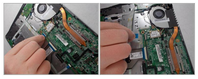
• Pull the blue tab on the ribbon cable to remove it.
