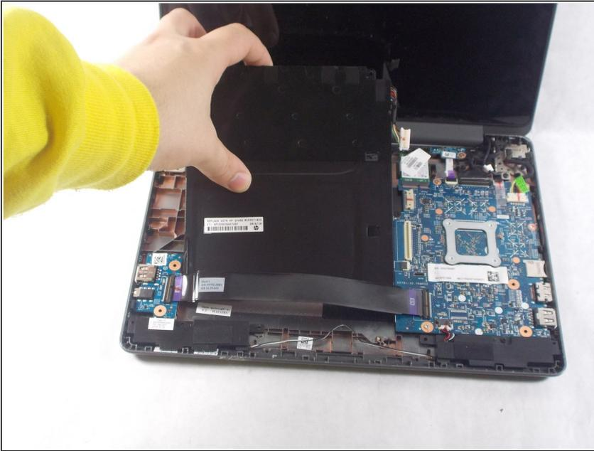
**⚠** There is a thick black wire strip that is going across the battery for a different part of the HP ChromeBook 11-v011dx. Be mindful when removing the motherboard so you do not damage this strip.
