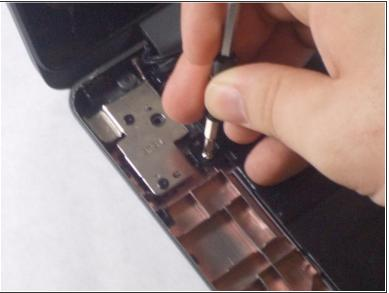
Remove three of the 1.3mm screws that keep the battery in place with a Phillips #0 screwdriver.
