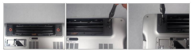
Use a JIS 1 screwdriver to remove (2) 7mm screws on the underside of the laptop near the battery bay.
