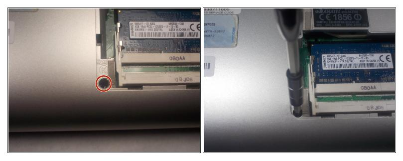
• Remove (1) 7.5mm screw with JIS 1 screwdriver marked by the letter "K" in the RAM bay.
