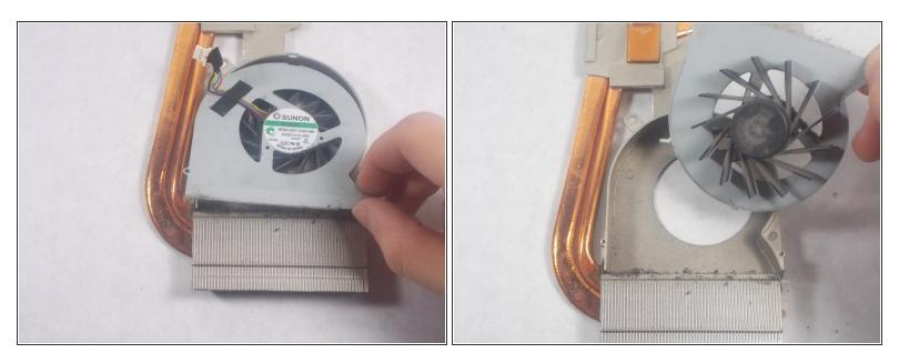
• Remove the cooling fan from the heat sink assembly by pulling it upward.
