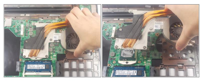
• Carefully pull the heat sink assembly upwards off of the motherboard after all the captive screws have been loosened fully.
