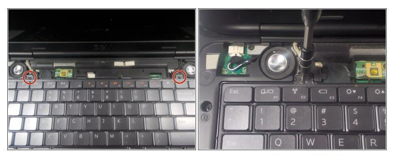
• Use a JIS 1 screwdriver to remove (2) 2.5mm screws located near the top of the keyboard.
