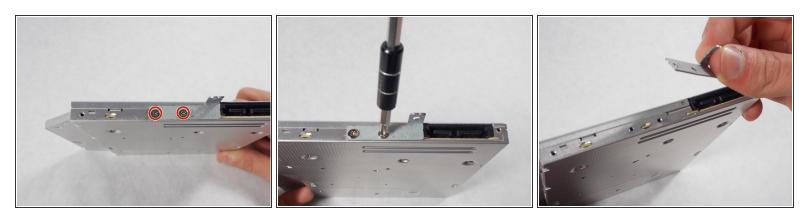
• Use a JIS 1 screwdriver to remove (2) 2mm screws on the drive's anchoring bracket.
