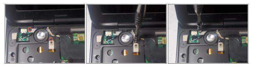
Remove (2) 4mm screws with a JIS 1 screwdriver that are holding down the left side display anchor.
