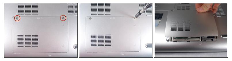
• Use a JIS 1 screwdriver to loosen the (2) captive screws from the panel.
