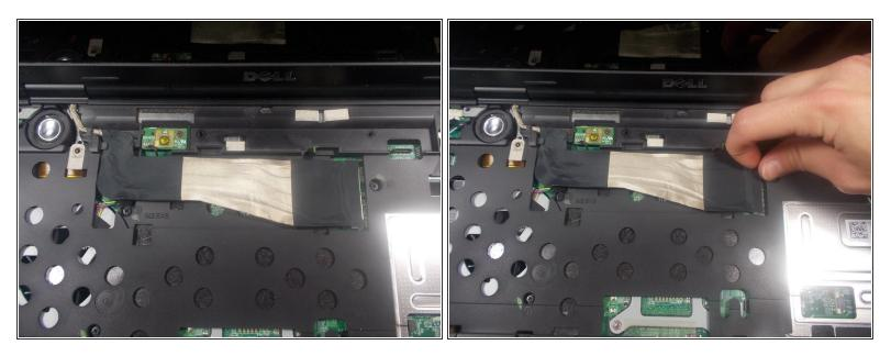
Disconnect the display ribbon cable by pulling the cable to the right by its sheathed plastic connector.
