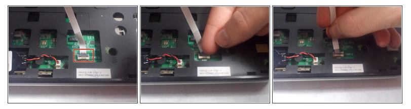
• Disconnect the track pad cable by flipping up the gray clamp and lifting the cable up.
