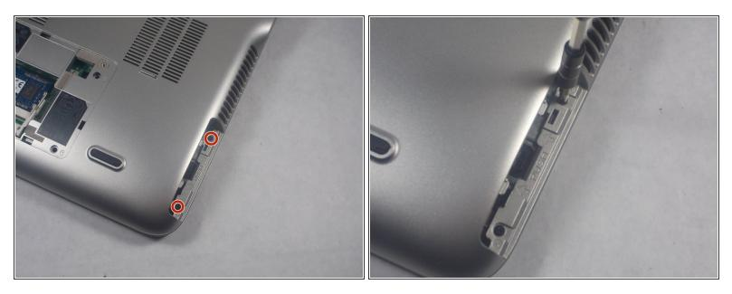
• Remove (2) 4.5mm screws with JIS 1 screwdriver marked by the letter "K"in the hard drive bay.
