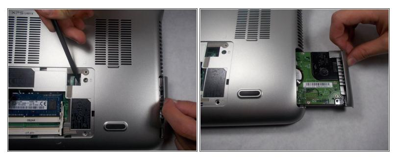
• Push the hard drive to the right with a spudger to unseat it from its socket while pulling out the hard drive with your other hand.
