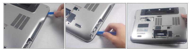
Separate the bottom cover from the top cover with plastic prying tool and finish lifting the bottom cover off.
