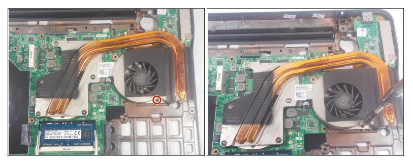
Use a JIS 1 screwdriver to remove (1) 4mm screw on the cooling fan assembly.
