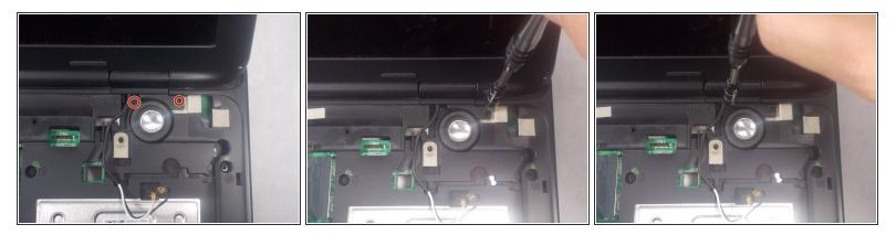
Remove (2) 4mm screws with a JIS 1 screwdriver that are holding down the right side display anchor.
