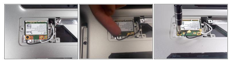
Disconnect the two wires on the mini card by carefully plucking them upwards by the metal contact points at the terminals.
