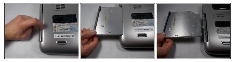
• Carefully pull out the optical drive from its bay.
