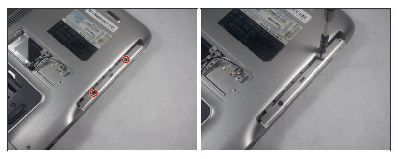
• Remove two 4.5mm screws with JIS 1 screwdriver marked by the letter "K" in the optical drive bay.
