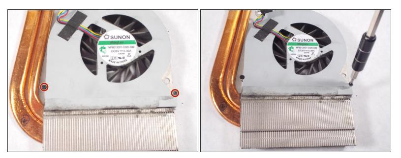
• Remove (2) 2mm screws on the sides of the cooling fan with a #00 Phillips screwdriver.
