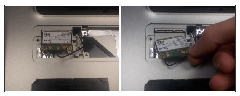
• Remove the mini card as it flips upward.
